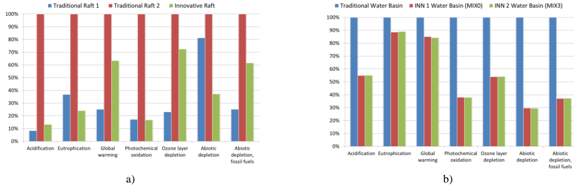
Figure 2. a) Comparative LCA of the Off-shore aquaculture raft; b) Comparative LCA of the Cooling tower water basin
