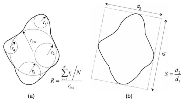
Figure 2. Definitions of (a) roundness,  $R$ , (b) sphericity,  $S$ , (adapted from [5]).
