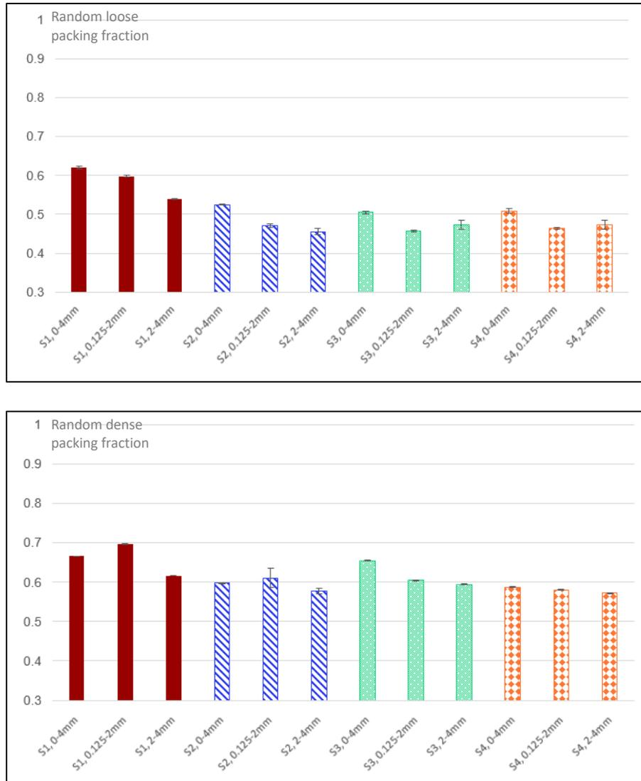
Figure 4. Random loose packing fraction (top) and random dense packing fraction (bottom) for the sands and various fractions.
