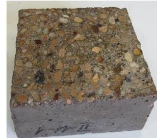
Figure 3. HP SCC (mix 2) sample after 28 freeze-thaw cycles
