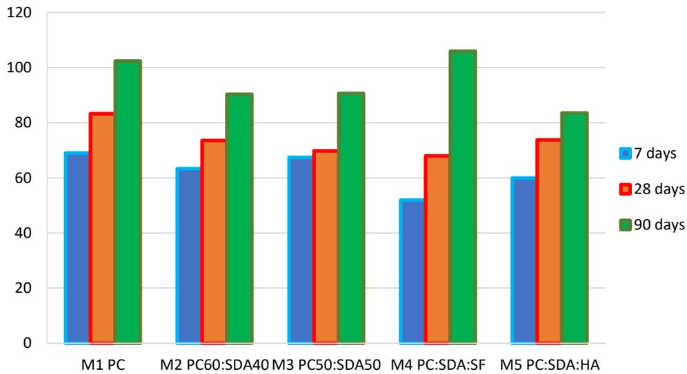
**Figure 2.** The Compressive Strength of Mortars
