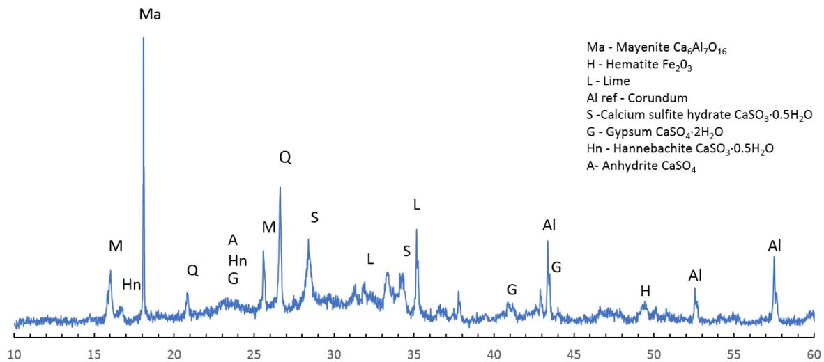
**Figure 1.** The XRD for SDA material used in the study
