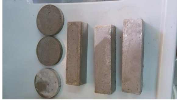
Figure 1. Samples used in the tests of physical and mechanical properties of hardened mortars
